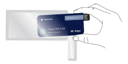
Open the outer transparant packaging bag and take the datalogger out of the package.
