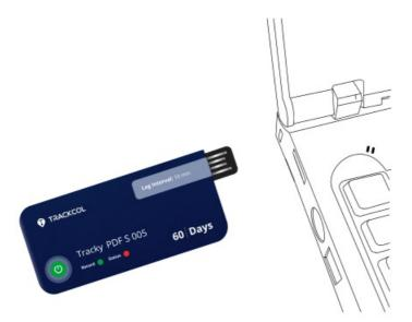
Insert the logger into the USB port of the computer to view the PDF/CSV report. The green and red LED will stay on until the recorder is removed from the computer.
