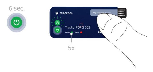
Press the start/stop (green) button and hold for 6 seconds. The red LED will flash 5 times. The recording has stopped.
