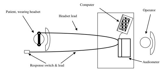
The patient is seated in front of the desk facing away from the operator. The patient wears a headset (see Section 3.6) and responds to test stimuli by use of a hand-held switch which is also connected to the instrument.
